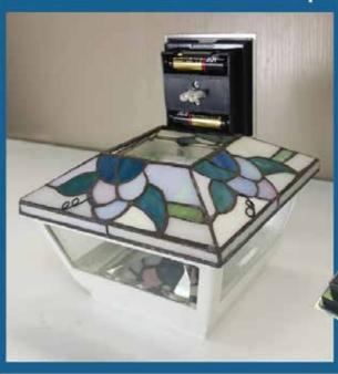
The solar collector simply lifts up from the glass topper. No need to remove entire light. You will now have access to replace batteries and or solar collector as needed.
